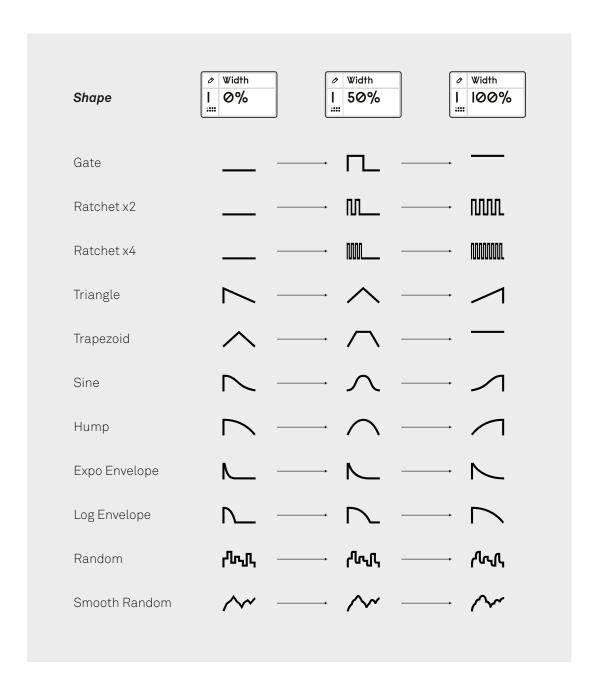
For random waveforms an additional slew parameter is made available. This smooths the edges of the random wave.
