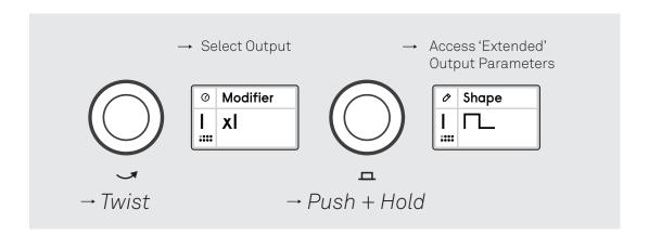
The various parameters can be cycled through and edited using the program knob just as when editing output modifiers. To exit back up to the main output modifier screen, click and hold the program knob again for just over 1 second.
